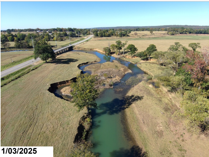
Embankment erosion upstream. Drone photo.
